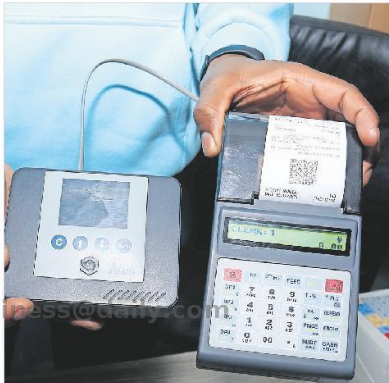
An electronic tax register machine for automatic transmission of tax data by businesses in Kenya. FILE
